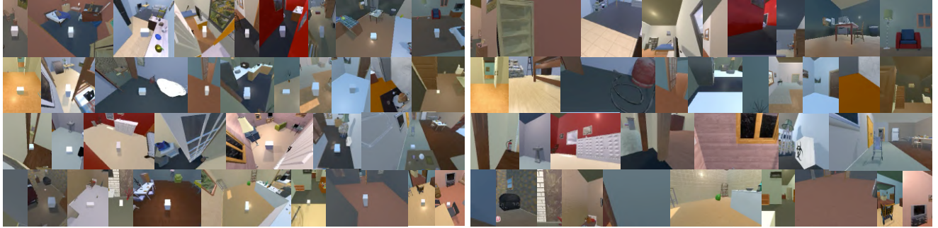
Figure 14. Random embodiments in the AI2-THOR simulator. Right column shows the egocentric view from the main camera and the left column shows a third-person view of the agent –white boxes indicate the robot colliders for visualization purposes only.
